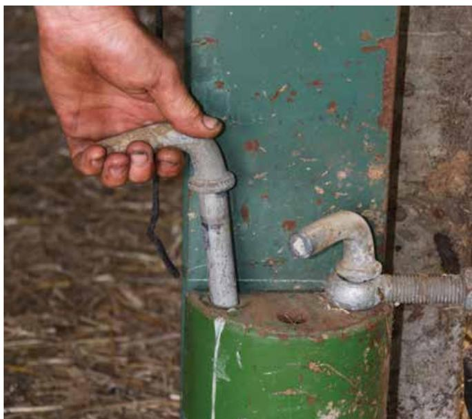
This adjustable gate hinge system is widely used on the farm to give an extremely flexible gate and penning system.
